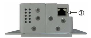
1. HDBaseT OUT: RJ45 port - Connect with receiver via a CAT5e/6 cable to deliver Audio/ Video signals with support for PoC from receiver. Note: The TPHD2-WP1 supports unidirectional PoC and cannot be used to power far-end receiver.
