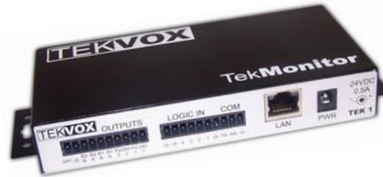
**TekMonitor** is at the center of TekPatrol. Each TekMonitor is an Ethernet-based, asset management tool providing equipment monitoring, security and control of audio visual devices. A TekMonitor maintains information about a device on its own and can send Email information about the device.
